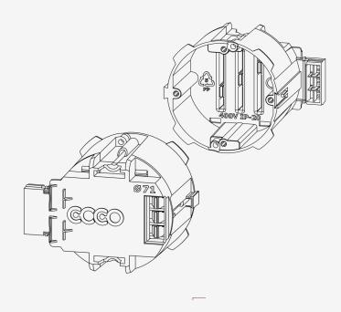
Installation box for hollow and concrete walls. Measurements according to the standard DIN 49073-1, for plate thickness 5-35mm. Standard distance between centers 71mm.
